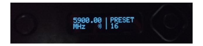
To select a menu header, you press the button on the left of the LED display and then using the joystick controller on the right side of the LED display, you can scroll through the menu headings: STATUS / CONFIGURATION / PRESET / UNIT
