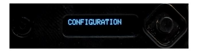
There are four menus heading under the CONFIGURATION menu: RF / VIDEO / AUDIO / DATA By pressing the joystick and scrolling down, you can select which menu you want to see. By pressing the joystick again, you will enter that menu.
