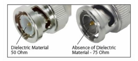
The HD/SDI Video input connector is 75 Ohms. Make sure that the video cable(s) are fitted with 75 Ohm connectors.
